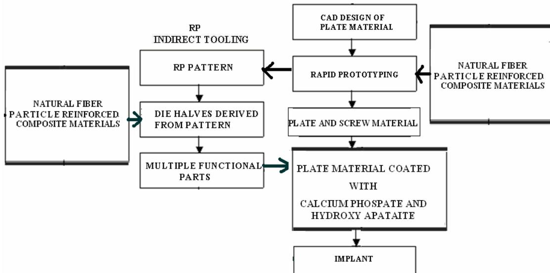
**Figure 7** Procedural steps followed to make a NFRPC plate and screw material using RP
