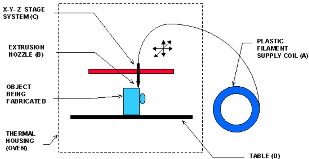
Figure 4 FDM Process representation diagram
